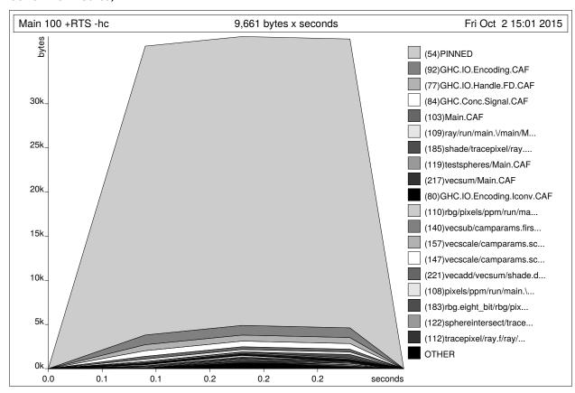
For example, here is a heap profile produced for the sphere program from GHC's nofib benchmark suite.
