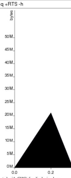
For example, here is a heap profile produced for the program given above in Section 5.1.1:
